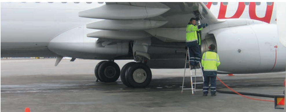
Aircraft on the apron being supplied with kerosene
